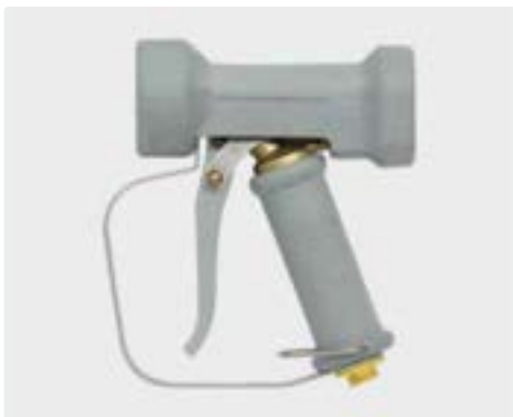
Spray gun with adjustable spray angle. Trigger guard. Max. 24 bar / 100 l/min / 50 °C
