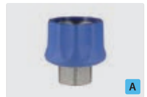
Coupling : F. Nickel-plated brass. Max. 250 bar / 150 °C
