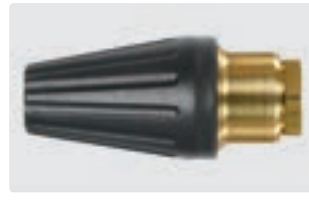
1/2" F. Spray angle 20°. 120 - 250 bar. Max. 100 °C
