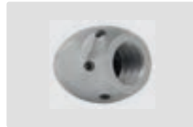
1/2" F. 6x 75° +1x 0°. 30-100 l/min. For \text{R} \text{D} 100-200 mm. Outside \text{D} 40 mm. \text{W} 281 g.
