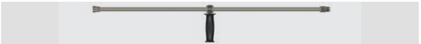
1/2" M. Lance with grip and sleeve 1/4" F NPT stainless steel without high pressure nozzle. Max. 600 bar / 150 °C
