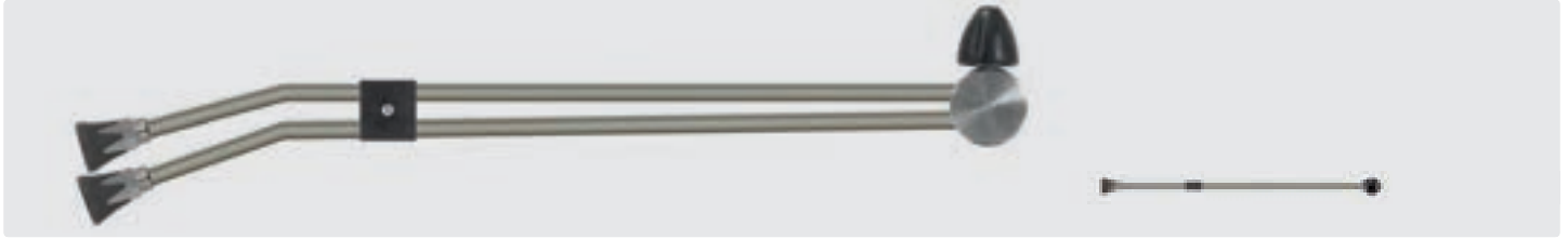
1/4" F. Lance with valve ST-53.2 on top and nozzle protector ST-10 with low pressure nozzle. Max. 400 bar / 150 °C
