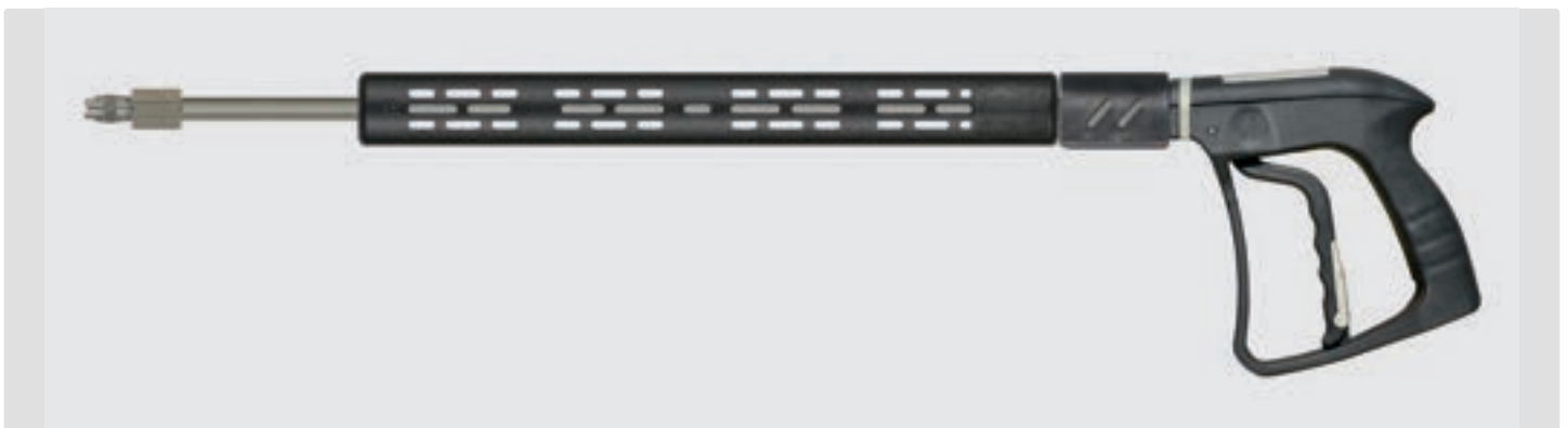
Professional steam gun ST-4000 with lance 500 mm stainless steel with vented handle ST-9 380 mm and steam low pressure nozzle made out of stainless steel. Max. 20 bar / 200 °C
