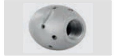
3/4" F. 6x 75° 3x 30° +1x 0°. 100-250 l/min. For \text{R} \text{D} 150-300 mm. Outside \text{D} 50 mm. \text{W} 1,367 g.
