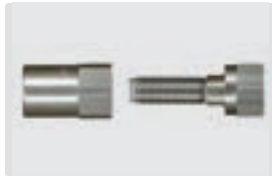
1/2" F with 60° cone. Stainless steel. Max. 50 bar
