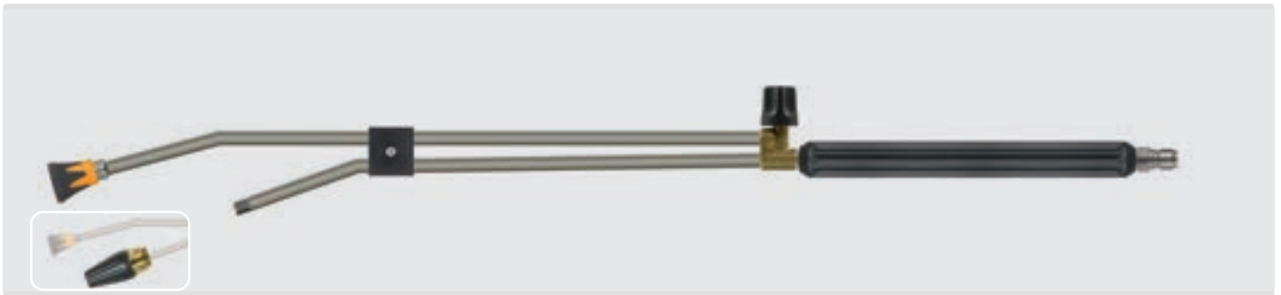
Plug ST-3100. Lance stainless steel, moulded handle 300 mm, valve ST-53 on top, nozzle protector ST-10 with low pressure nozzle and 1/4" M thread for rotating nozzles. Lance without rotating nozzle. Max. 250 bar / 150 °C
