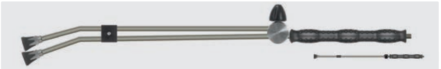
1/4" M. Lance with moulded handle ST-29 Cool & Compact, valve ST-53.2 on top and nozzle protector ST-10 with low pressure nozzle & thread 1/4" F. Max. 400 bar / 150 °C
