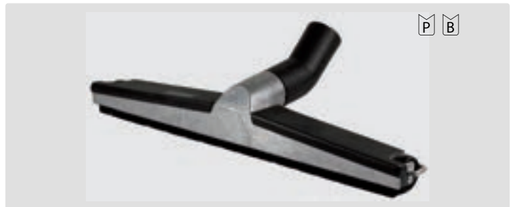
All-purpose nozzle GRD 450. Vacuum tool with brush strips, rubber lips and height adjustable rollers. Aluminium. For all carpets and hard covers
