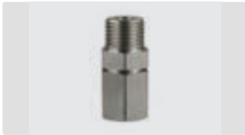
1/2" M : 1/2" F. Stainless steel. Max. 350 bar / 90 °C
