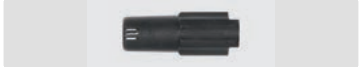
1/4" F. Housing black. Nozzle and seal kit ceramic. Adjustable spray angle. 100 - 250 bar. Max. 80 °C
