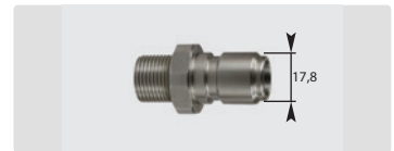
Plug : M. Stainless steel. 60° cone. Max. 250 bar / 150 °C
