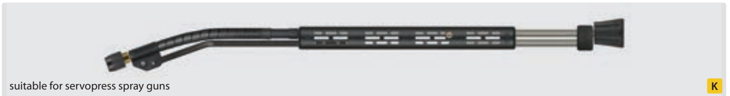
M22 F swivel. ST-85 Push & Pull lance with ergonomic swivel screw coupling suitable for servopress spray guns. Max. 210 bar / 150 °C
