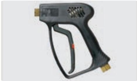
Professional gun. Max. 275 bar / 45 l/min / 150 °C
