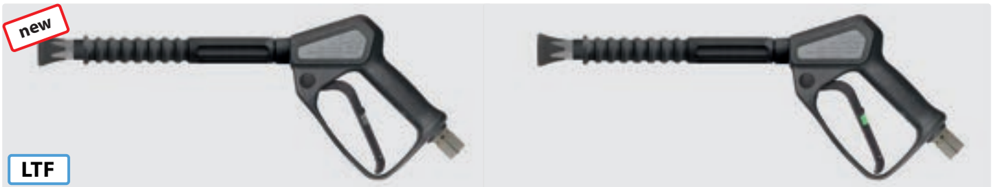
Professional low pressure foam lance with patented LTF technology. Gun ST-2620 with 300 mm insulated lance and nozzle protection ST-10 with low-pressure nozzle 9040. Max. 125 bar / 80 l / min / 150 °C
