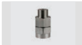
3/8" M : 3/8" F. Stainless steel. Max. 500 bar / 90 °C
