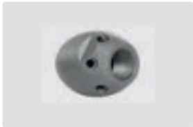
1/4" F. 6x 75° +1x 0°. 20-50 l/min. For \text{R} \text{D} 50-100 mm. Outside \text{D} 30 mm. \text{W} 127 g.
