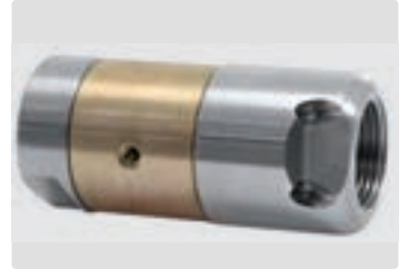
3/4" F. rear jets. 3 side jets. Outside \varnothing 38 mm. 554 g.
