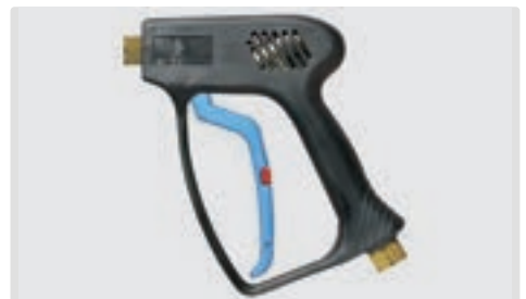
Professional gun. Freeze stop version. Max. 275 bar / 45 l/min / 150 °C
