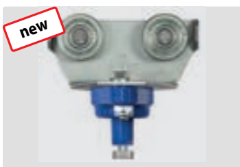
For C-Rail 32 x 30 mm. Load capacity 20 kg. Rollers with ball bearings.
