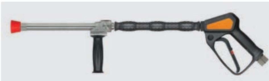
1/2" F. Stainless steel. Longcast lance 350 mm with insulation ST-29 Cool & Compact 330 mm, gun ST-2320, grip aside and nozzle protector made out of plastic without nozzle. Max. 150 bar / 80 l/min / 100 °C
