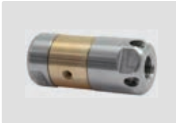
1/4" F. rear jets. 3 side jets. Outside \varnothing 30 mm. 314 g.
