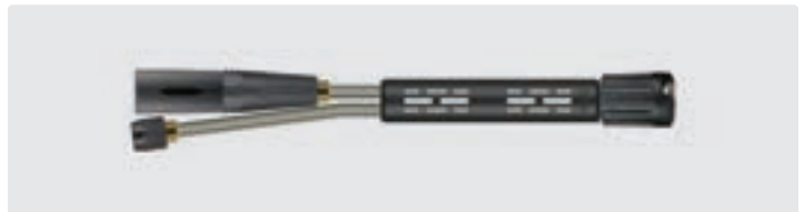
Twin foam lance with vented handle ST-9 205 mm, change-over valve ST-58, nozzle protector without tip and foam head ST-75.1 without nozzle. A foam injector is required. Max. 350 bar / 45 l/min / 100 °C
