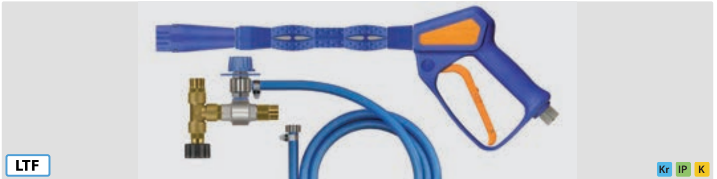
easywash365+ foam set: easywash365+ foam lance standard with foam head ST-75, injector ST-160 (M22 F and 2 x M22 M) with metering valve ST-161, suction hose 1,000 mm and suction filter ST-32. Max. 310 bar / 90 °C
