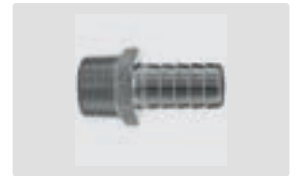
Hose barb 3/4" M. 60° cone. Stainless steel. Max. 15 bar
