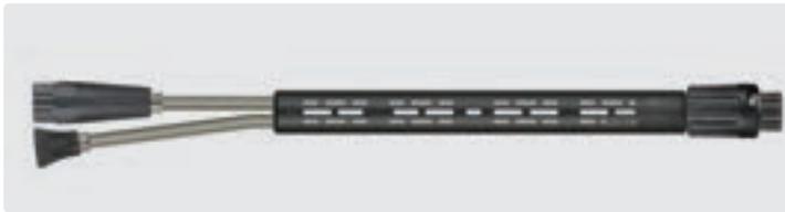
Twin foam lance with vented handle ST-9 380 mm, change-over valve ST-58, nozzle protector ST-10 without nozzle and foam head ST-75 with nozzle. A foam injector is required. Max. 350 bar / 45 l/min / 100 °C
