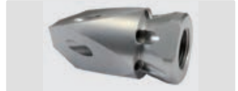
350 bar. 3/8" F. For tubes > 50 mm. Lateral front jets with hardened stainless steel nozzle inserts
