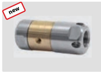
3/8" F. 4 rear jets. 3 side jets. Outside \varnothing 30 mm. ☒ 307 g.
