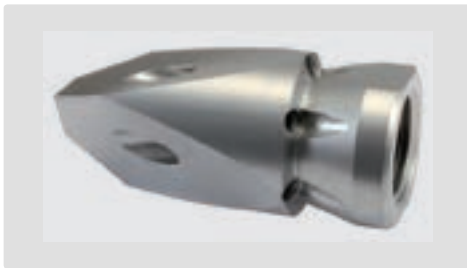
350 bar. 1/2" F. For tubes > 60 mm Lateral front jets with hardened stainless steel nozzle inserts
