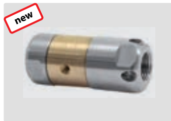
3/8" F. 4 rear jets. 3 side jets. Outside \varnothing 30 mm. ☒ 305 g.
