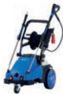
The MC 7P FA is equipped with the renowned, industrial class, C3 pump based on a tough 4 piston pump construction, double roller bearings, flow activated control system and 1450 rpm motor for long lifetime and low noise level. Ideal for the toughest of industrial applications.
