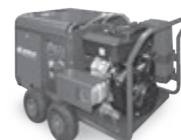
HDB/HDD Series Mobile Hot Water High Pressure Cleaners with petrol or diesel engine for professional users, 16 - 17 l / min, 200 - 300 bar
